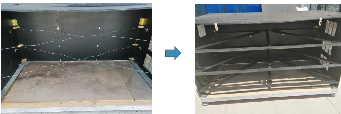
Fig. 14. Macroalgal dryer internal structure before (left) and after the technical improvements (right).
