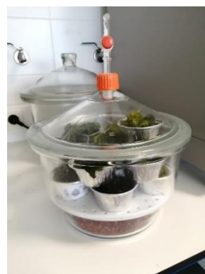
Fig. 9. Ulva samples extracted from dryer trials in a commercial oven to calculate measure moisture content (left) and post storage in a desiccator silica gel until being weighted
